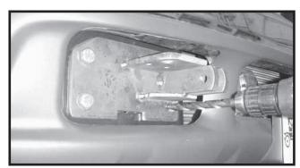
**5.** Using pull pod as template, drill 1/2" holes on inside holes of pull pod through bumper. Install 1/2" x 1-3/4" bolts, 1/2" flat washers, 1/2" lock washers, and 1/2" hex nuts and tighten.
